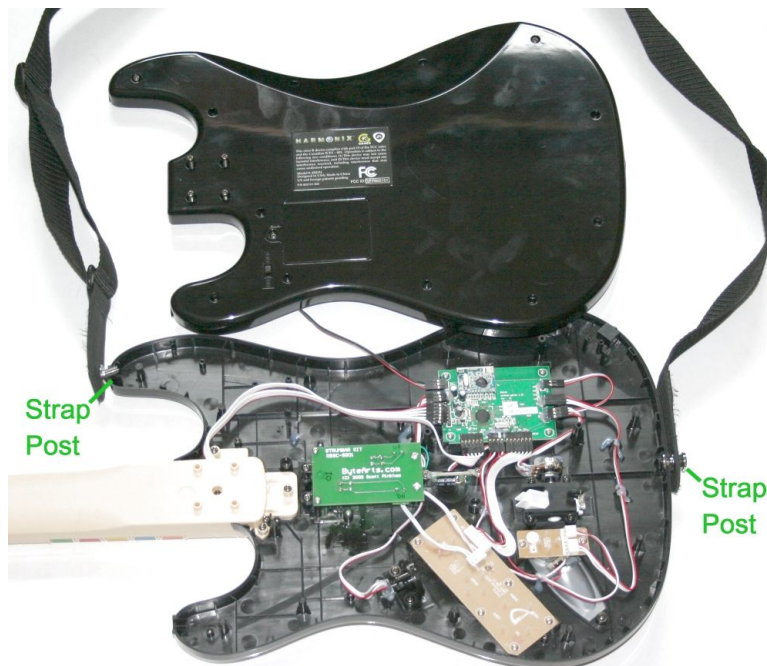
Guitar with back cover removed (the Strum Fix is already installed in this photo).
